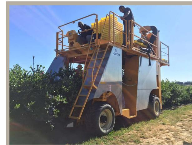
In a study done by Takeda et. al., this machine harvester was developed to address the issues of increasing labor costs, decreasing labor availability, and fruit quality. Not only does it vastly decrease the amount of picking time versus hand-harvesting, but it increases the amount of viable fruit collected by 3.5-15 times (g/min) versus other machine harvesting methods.
